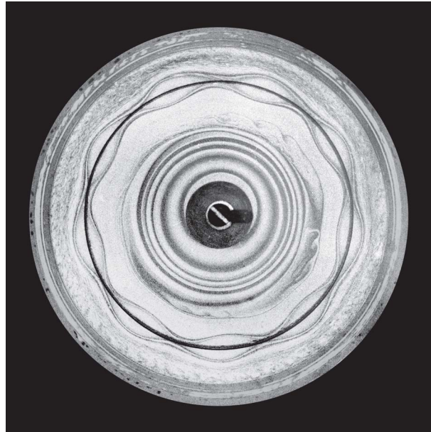
Figure 2. Dynamics of a circular shear visualized by a soapy water membrane. Photo Yves Couder.
